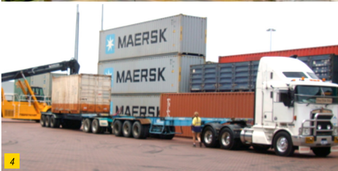
Figure 3: The Toll intermodal freight forwarding facility in Kewdale | Figure 4: A reach stacker in action loading a double road train Figure 5: ITV's are used to transfer containers from the rail terminal directing to Toll's facility (anti-clockwise)
