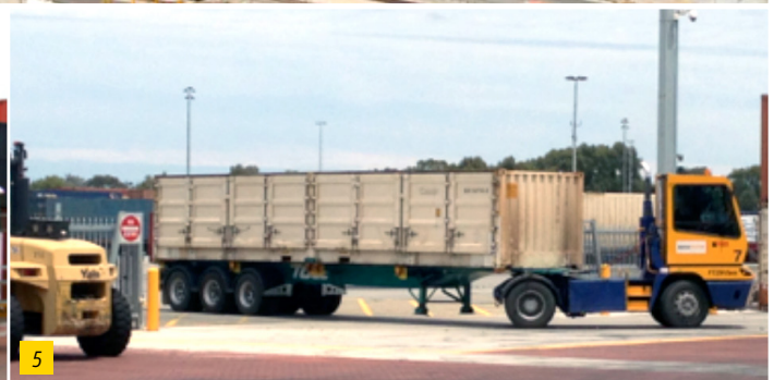
Figure 3: The Toll intermodal freight forwarding facility in Kewdale | Figure 4: A reach stacker in action loading a double road train Figure 5: ITV's are used to transfer containers from the rail terminal directing to Toll's facility (anti-clockwise)
